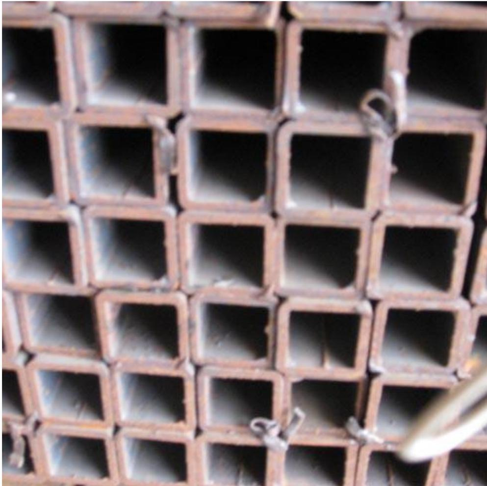
The flat square surfaces of RHS has the ability to ease construction, and they are sometimes preferred for architectural aesthetics in exposed structures, but circular Hollow Structural Sections are becoming more popular in exposed structures for the same reasons.
