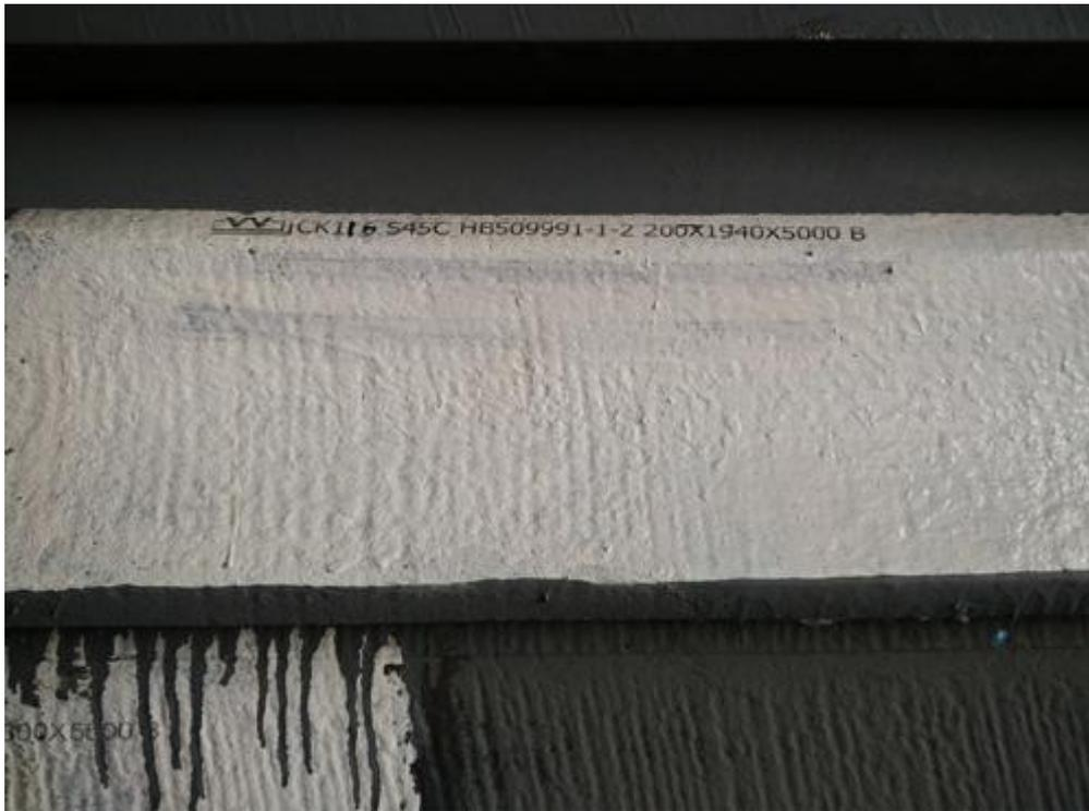
The carbon content of the steel is above 0.4%, and its wear resistance is excellent, but its ductility is reduced. Quenching is easy to deform and crack. Therefore, heat treatment is very important, and it must be quenched immediately after tempering to avoid temper brittleness. The cutting properties of this kind of carbon steel can be improved by spheroidizing the steel.
